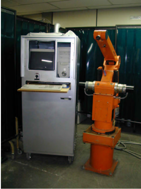
Fig. 13: Controller enclosure front view.
