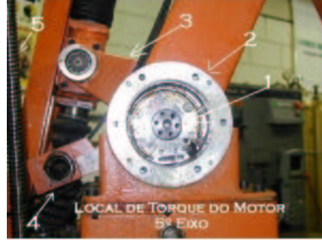
Fig. 5: Screw (5) and lever (3) for actuating joint 2, lever for actuating joint 3 (4) and coupling for joint 5 actuator (1).
